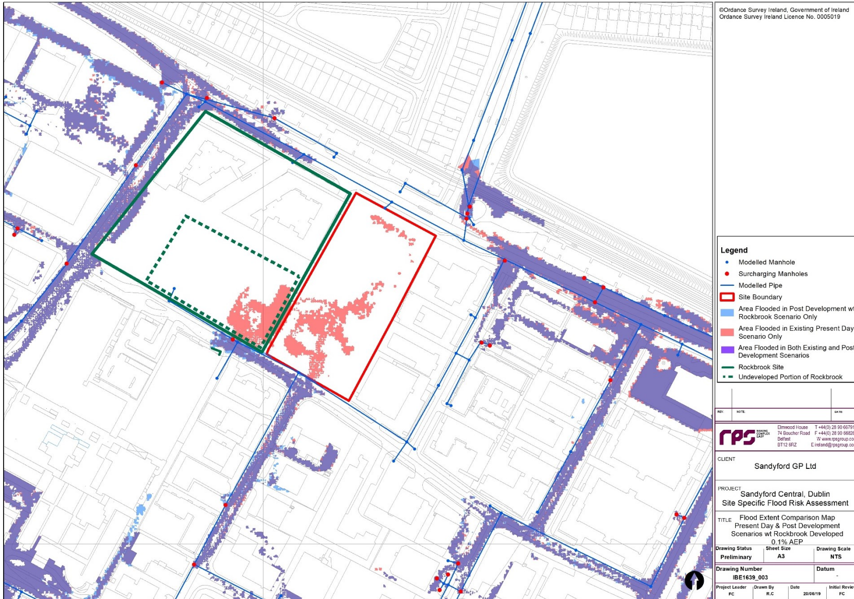
Figure 7.5 Comparison of Pre and Post Development Scenarios 0.1% AEP Extents (with Rockbrook site developed)
