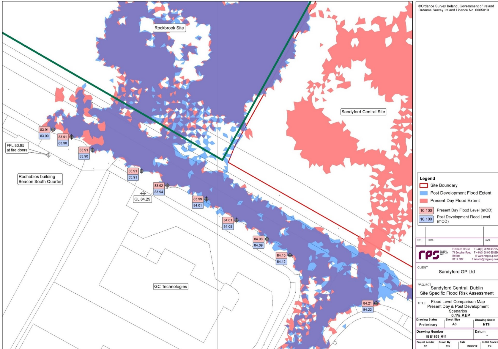
Figure 7.4 Comparison of Levels Pre and Post Development Scenarios 0.1% AEP
